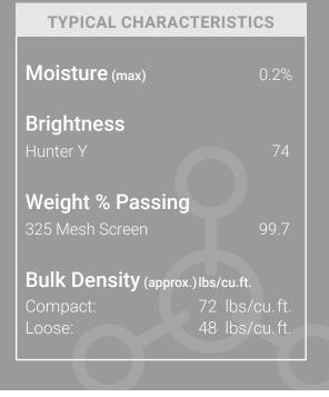
GLC CalPro<sup>™</sup> 1006 is a six micron product that consistently provides the chemistry and physical characteristics you need and can rely on. It is sourced in the U.S. and produced in an ISO 9001:2015 certified facility.
